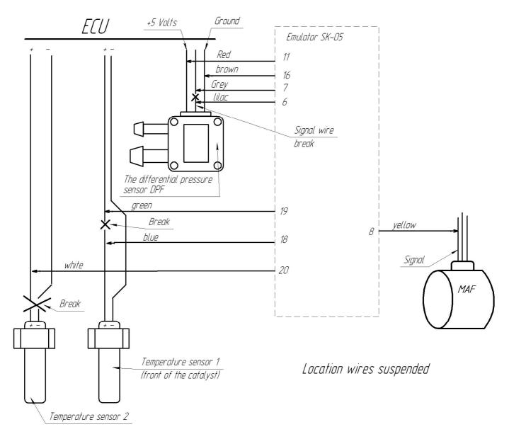
In Toyota/Lexus the yellow wire is connected to signal wire of the flow meter. The voltage of signal wire should change with change of engine speed:
